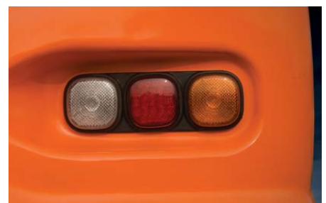
Stop lamp (LED type) As stop lamp in LED type is adopted, life and recognition have been improved considerably compared to the existing standard filament bulb. Furthermore, the fast lighting speed contributes to prevent accident.
